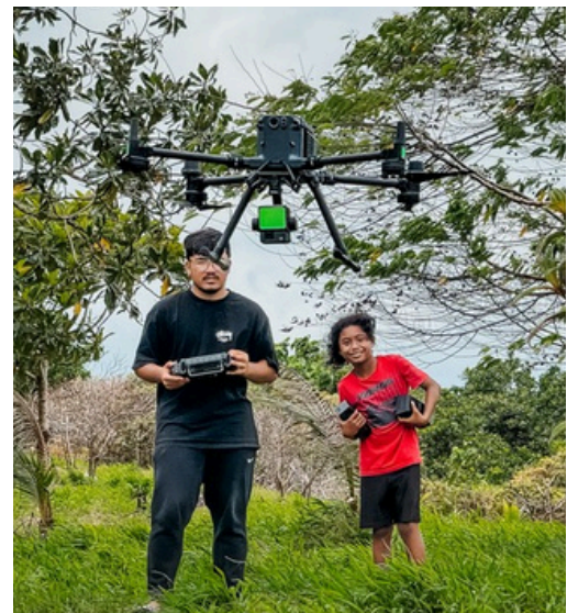
Thomas Torres II operates a drone equipped with a LiDAR sensor during a mapping mission in Aimeliik State, Palau
