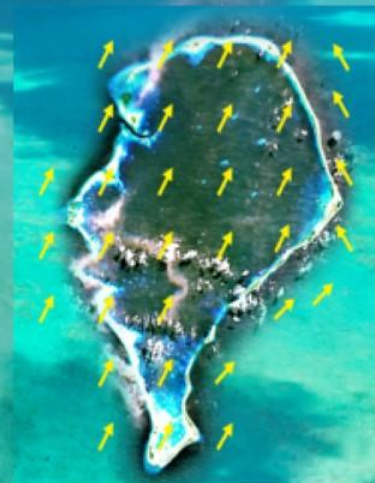
Wave properties retrieval : wavelength, wave direction
