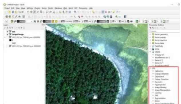
Figure 2: OTB as an application framework within QGIS highlighted in red box
