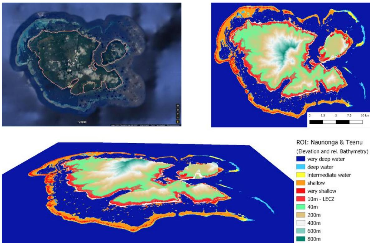
Figure 1: Example of the merged DEM and the relative bathymetry layer. Presented as an example here are the relatively small and remote Islands of Naunonga and Teanu (Solomon Islands).
