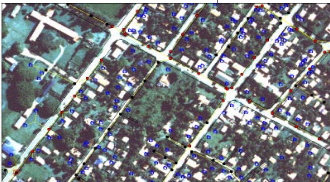
Figure 1: GIS display of TEPB; poles, lines and customers as top layers, a rectified aerial photograph as backdrop.
