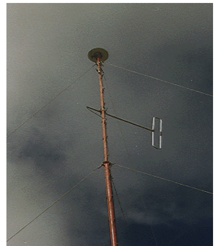
Figure 2: Below the GPS antenna a radio communication antenna is fixed on the pole
