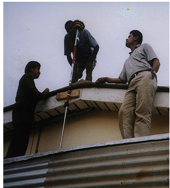
Figure 3: To avoid high costs of a conventional survey the antenna position was determined by using the location of trigonometric points. The picture shows Litea Biukoto (SOPAC) with Valimani Latilevu and Joai Duikovo (MSD-Forestry) during the field work.
