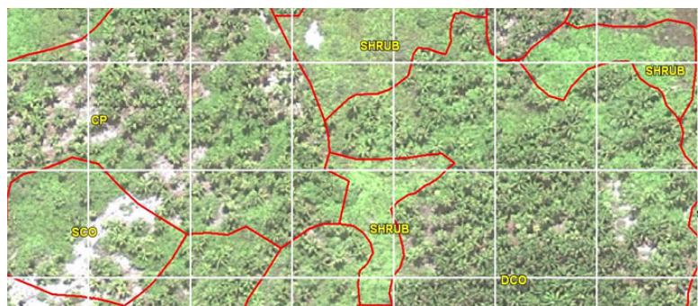
Figure 01: Stratification of coconut palms on very high resolution image data. DCO = dense coconut, CP = coconut plantation or medium, SCO = scattered coconut, the 50 x 50 m grid helps the interpreter
