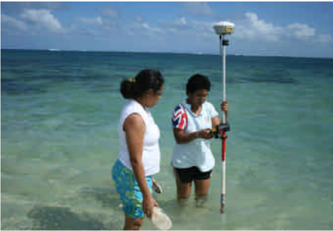
Figure 05: Some lines were surveyed in the water, where the operator tried to walk in the same water depth to best capture a contour line.
