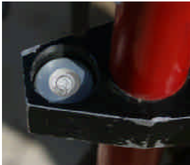
Figure 04: The spirit level mounted at the side of the survey pole indicates if the pole is in correct vertical position.
