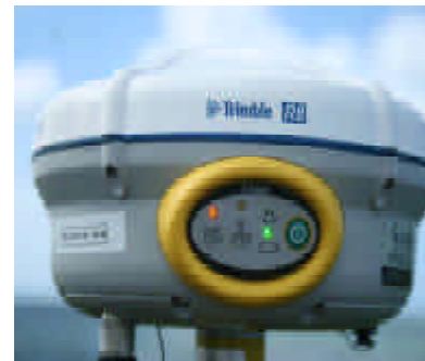
Figure 02: This base station unit contains the GPS antenna, the GPS receiving unit, the VHS transmitter and the battery.
