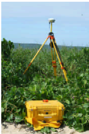
Figure 01: Base station in the centre of the sandbank of the Suva reef. From there it can transmit the position data for more than 1 km. (The transmission antenna pointing downwards on the left side of the instrument). The tripod position is marked with a peg for follow up surveys.
