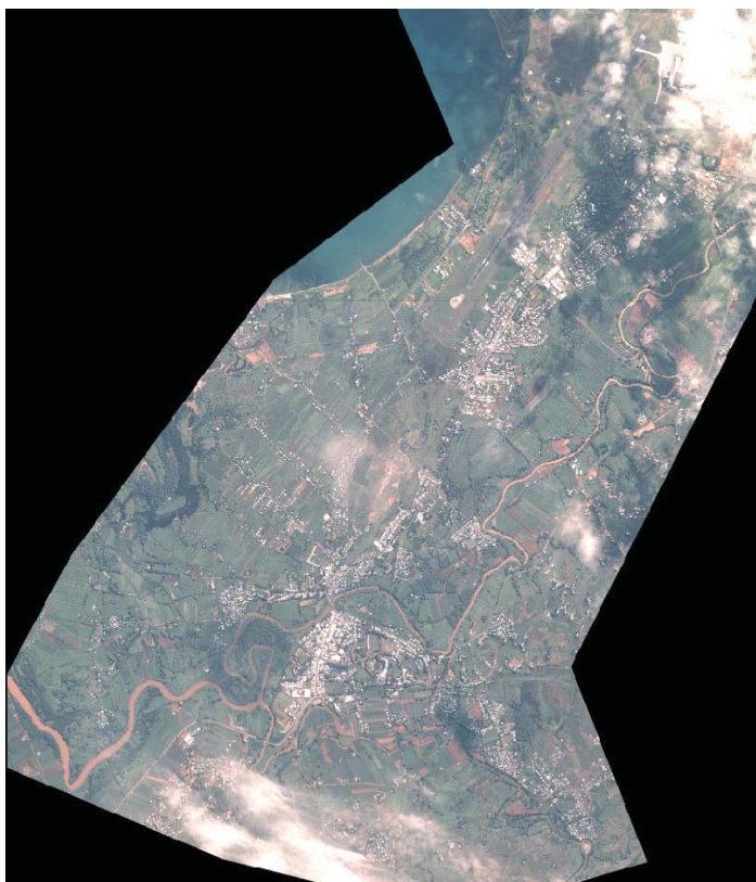
Figure 02: Pan-sharpened Quickbird Image data recorded over a period in 2006 with 60cm resolution. This image data was used as reference to rectify the radar data and to digitise the location of houses and infrastructure
