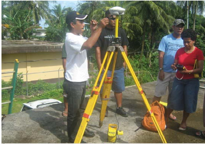
Figure 05: Setting up the base station on a known point
