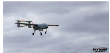
Fixed wing UAV ideal for capturing images of larger areas
