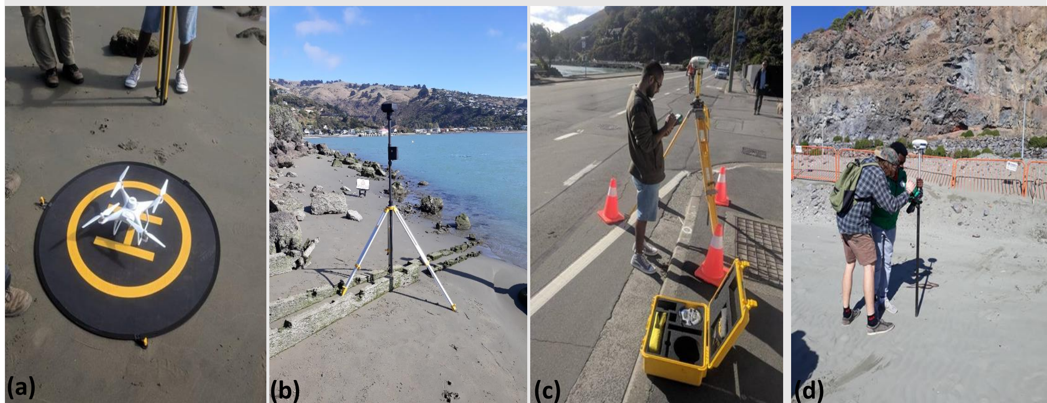
Figure 2 : (a) Phantom 4 RTK drone used for image capture (b) D-RTK 2 Mobile Station (c) GNSS base station set on a known bench mark (EKNU) for RTK profiling (d) GNSS Rover used for collecting profile data
