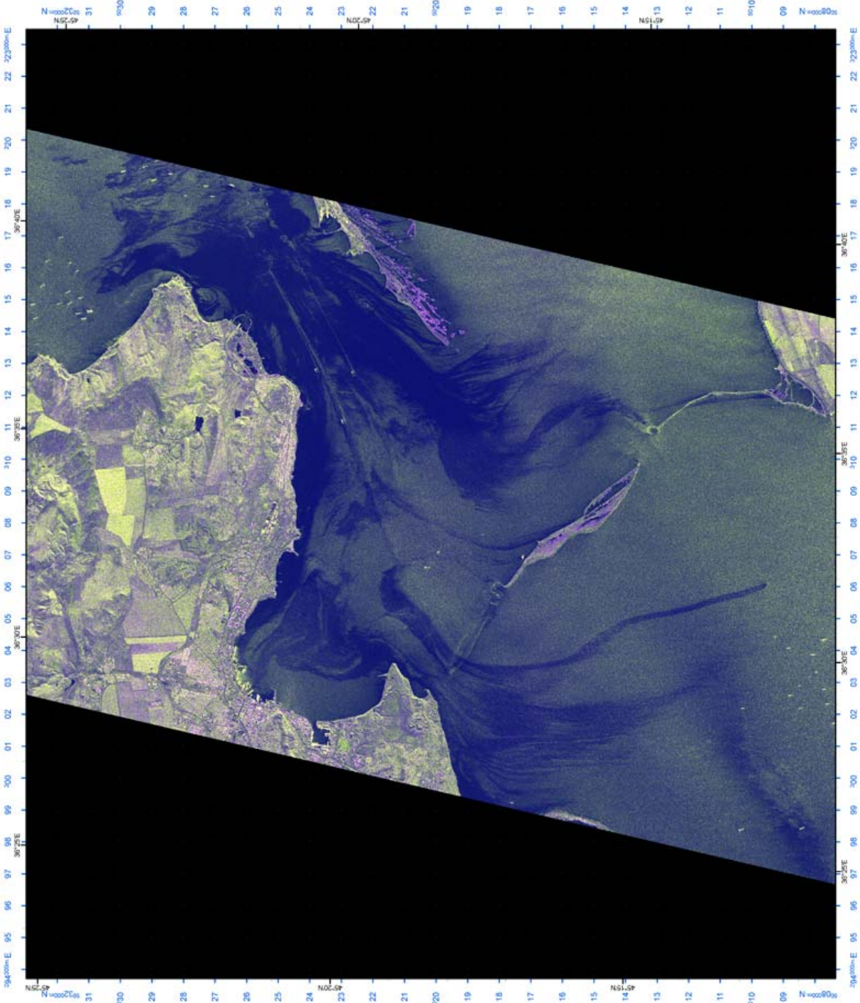
TerraSAR-X acquires oil slicks in the Black Sea - Nov 16 2007: The StripMap image acquired 5 days after an oil tanker broke into two pieces shows massive oil slicks drifting on the surface. 3m resolution / dual polarisation.
