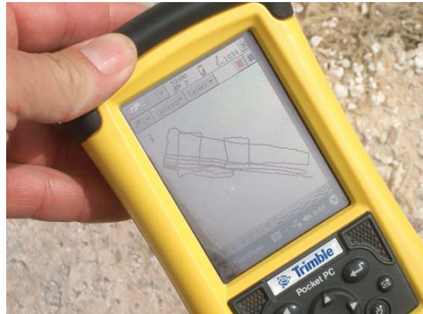
Figure 1: While following the contour lines at the beach the operator can monitor the survey on the display.
