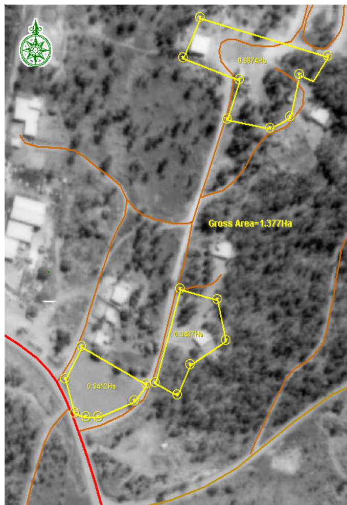
Figure 5: GIS display of aerial photograph after rubbersheet rectification and import to MapInfo.
