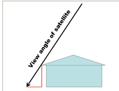
Figure 1: A roof corner as reference image point on the image data and during the survey. To determine the height position the distance between roof corner and antenna and the distance between roof corner and ground has to be measured.
