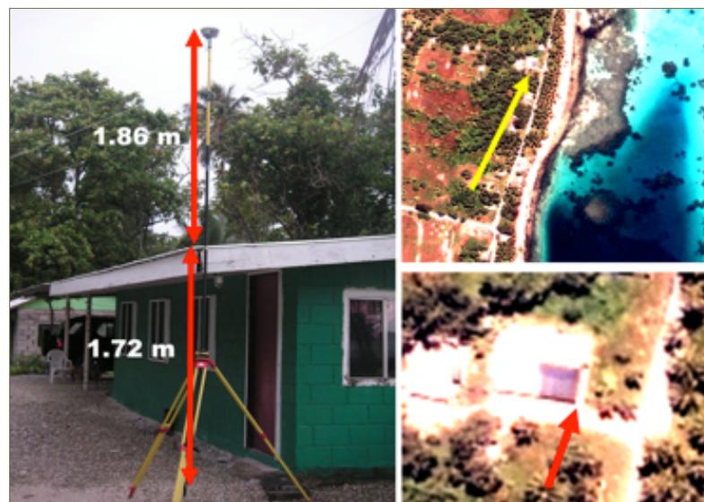
Figure 2: The distance between ground and roof corner has to be known to calculate with the view angle the displacement of the RIP.
