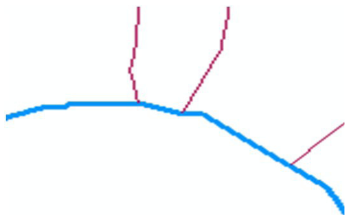
Figure 07: The existing stream lines are then extended and snapped to the new stream centre lines.
