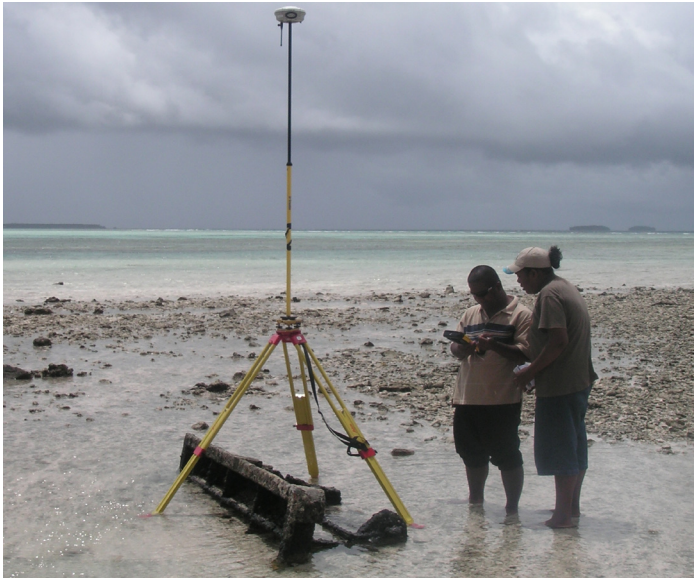
Figure 01: Local base station established on a engine block at the beach. The GPS antenna is mounted on a pole to increase the height and subsequently the field of view.
