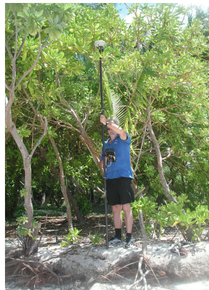
Figure 05: Mounting the rover on a 4m pole allowed GPS receiving under thin vegetation cover.
