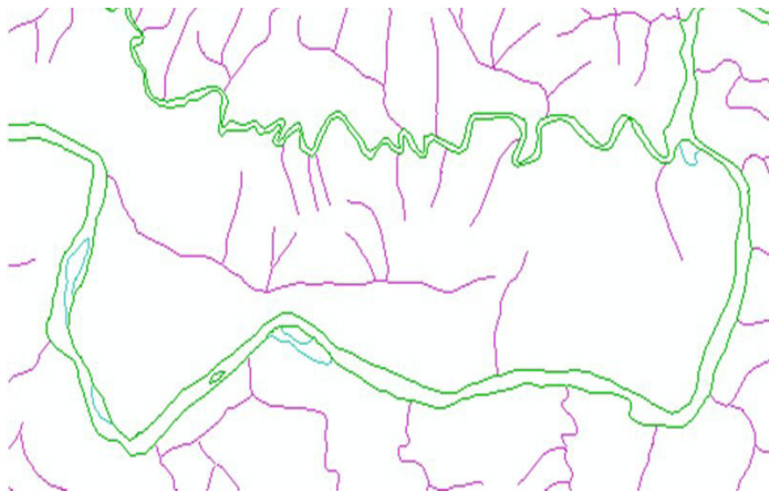
Figure 03: Two lines were used to represent the banks of wider streams and rivers.
