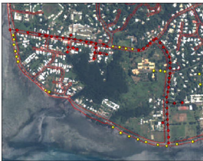
Figure 1: FEA vector data of street lights, overhead lines and power poles. The map backdrop is a 1:10,000 IKONOS multispectral image.
