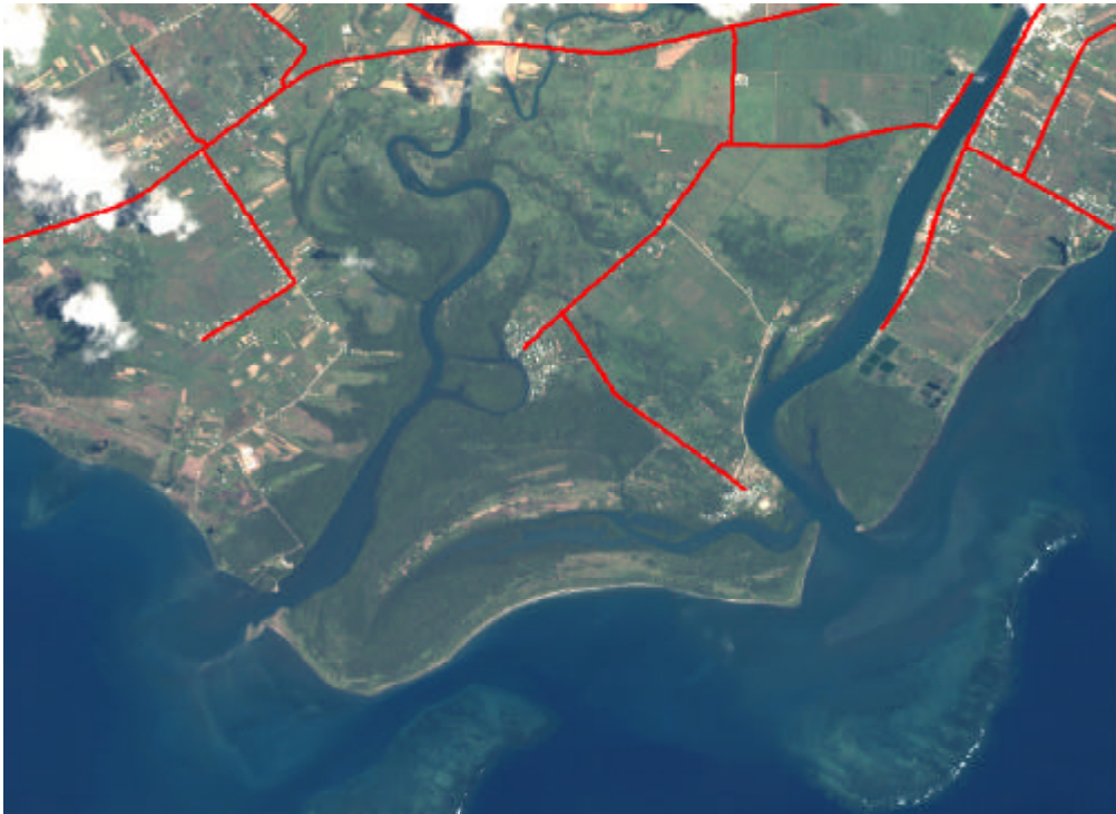
Figure 1: Multi-spectral IKONOS image data after image rectification to Fiji Map Grid. The DGPS surveyed road network (red overlay) provided by PWD was used as reference. The image shows Pacific Harbour at the South Coast of Viti Levu, Fiji
