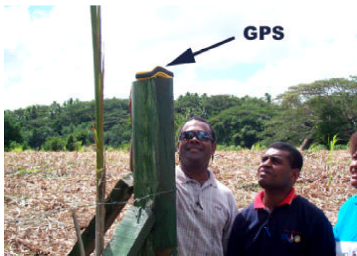
Figure 1: Position recording of a fence post used as boundary marker in a corner of a residential plot, which has to be separated from agricultural lease area .
