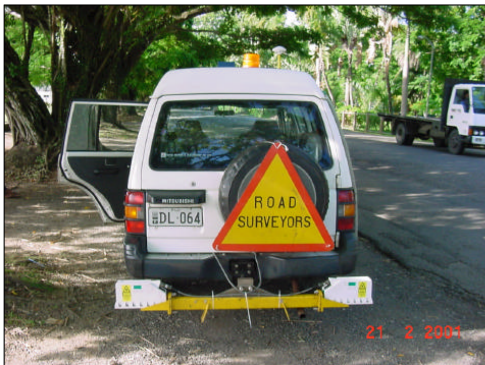
Figure 1: Vehicle used for road condition survey including GPS survey
