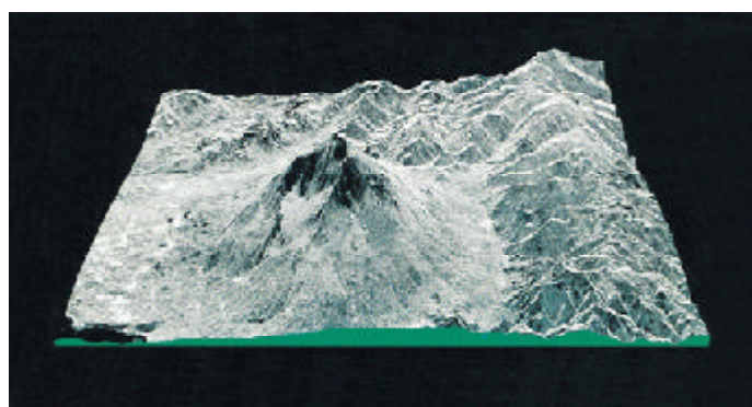
Figure 4: Digital terrain model image of the ETNA volcano built from ERS SAR data by ESA; with the ASAS in the ENVISAT, even better data is expected.
