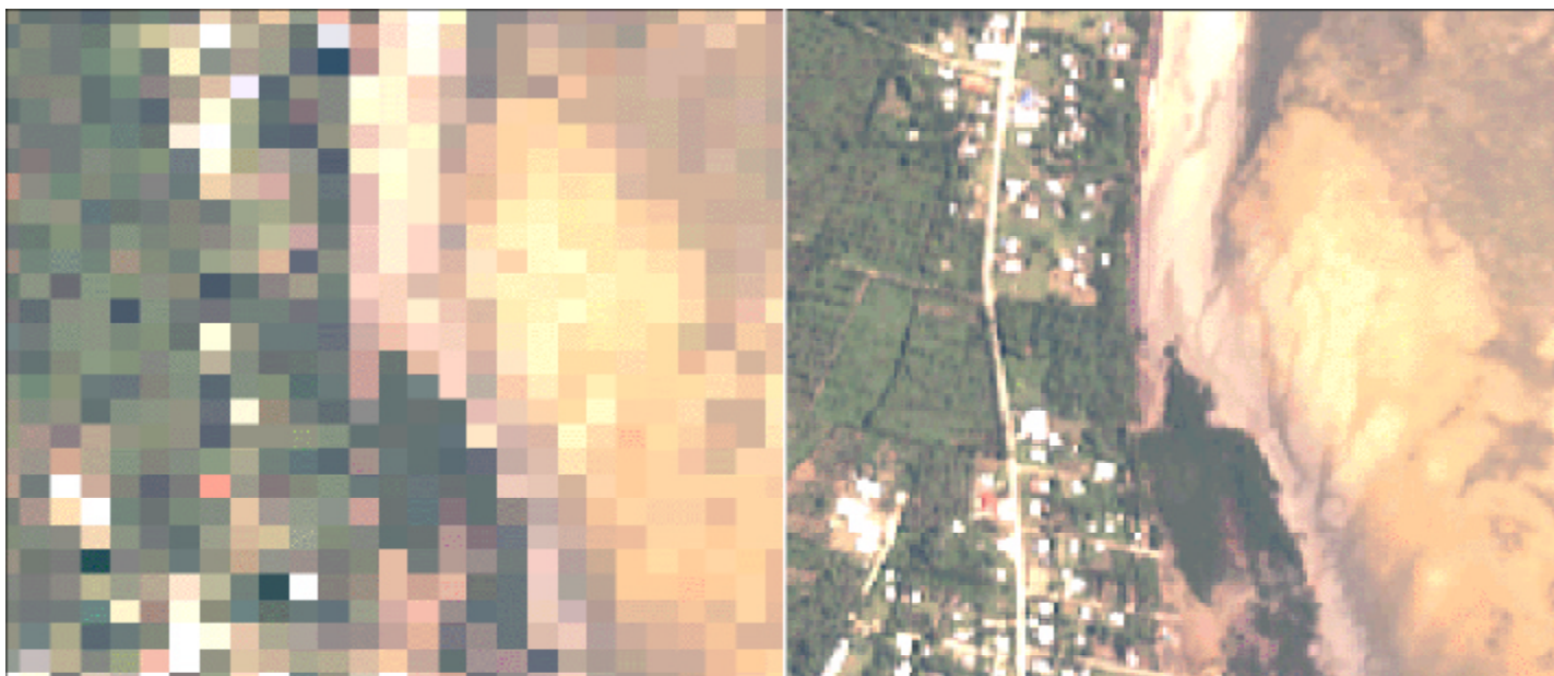
Figure 1: Left, Landsat image data with 30m resolution which does not allow to map at larger scale than 1:50,000. If zooming in further, the image information do not increase. Right, the same area recorded with multispectral 4m IKONOS data. Single trees, the shape of the houses and small tracks are visible. Such image backdrop is ideal for thematic mapping at 1:10,000 scale as required by utilities for GIS image backdrop.
