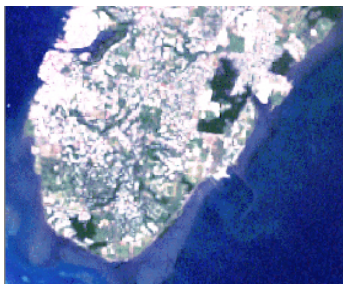
Figure 2: The image shows the bands blue, green and red of a part of a Landsat TM scene recorded in 1999 from Suva Peninsula. The image was geometrically rectified and resampled to 25m resolution.
