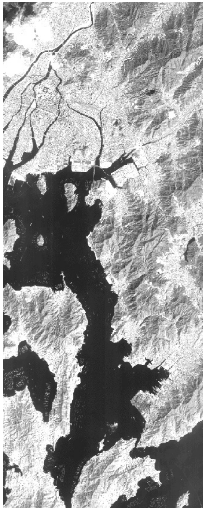
Figure 2: The image size received from ISI is 7,000 x 14,000 pixels equivalent to 12,5 x 25 km as the pixel size is 1.8m (area coverage see Figure 4) The customer pays $US 10 per km 2 and determines the image size with a minimum data purchase of $US 1000.
