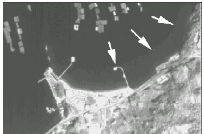
Figure 6: Water depth is difficult to see in panchromatic images. However, employing contrast enhancement shallow water can be delineated from more deep water (again, if the print comes out nicely).
