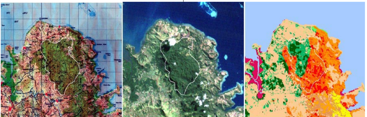
Figure 5: An example of GIS backdrop application in Forestry. The area outline e.g. a proposal for forest management under FSC regulations is first digitised using the topographic map backdrop. Then, the polygon is displayed over the satellite GIS backdrop to see if the area is still stocked by forest. Finally, the Forest Type / Forest Function GIS backdrop shows, that the main part is protection forest, which limits the forest management.
