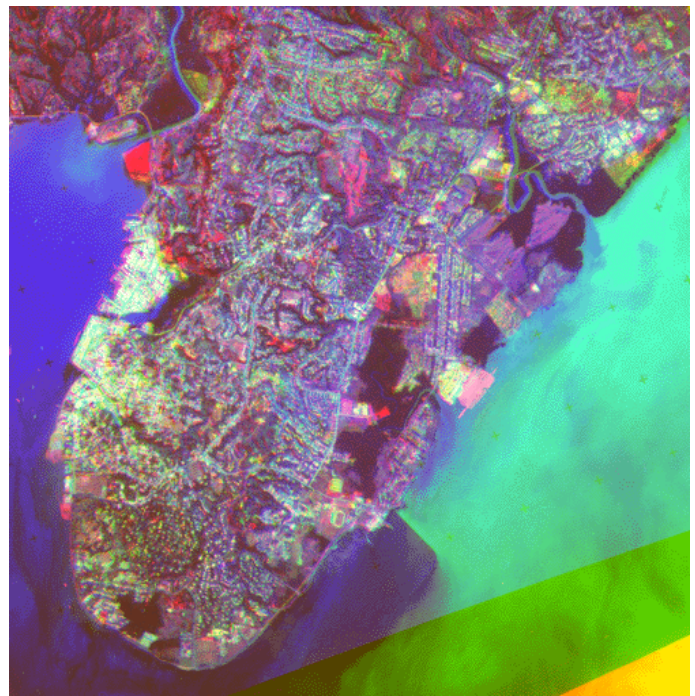
Figure 1: The change detection image of Suva peninsula: Aerial photographs recorded in 1973, 1986 and 1994 have been scanned, geometrically corrected and combined to one colour image as described in the text and by Figure 2.
