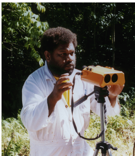
Figure 4: The Ledha-GEO instrument tested by Samueala Lagataki Officer of the Inventory Division of Fiji's Forestry Department. For good reading of upper diameters the use of a tripod is recommended.
