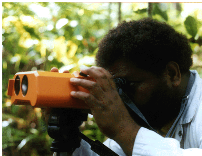
Figure 5: The operator focussing on the tree with the instrument's optic (right eye). At the same time, information of the database is displayed for the left eye. He operates with his right hand the measurement and with his left hand the database.
