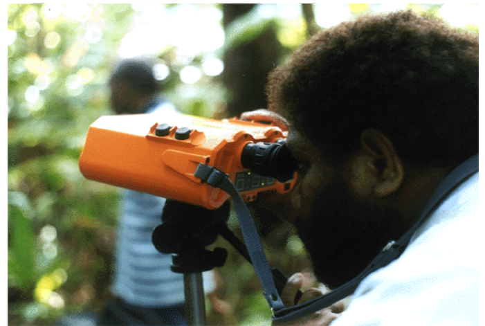
Figure 3: The right two buttons of the instrument control the measurement while the left ones are used to type in or select the tree number out of the internal database. On the front side different menus to measure the tree distance, tree height, compass bearing or tree diameters can be selected.
